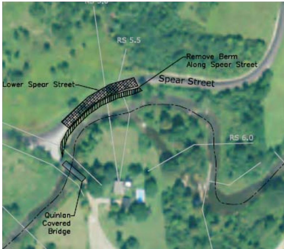
Figure 25. Alternative schematic of lowering berm and Spear Street to the north of Quinlan Bridge.
