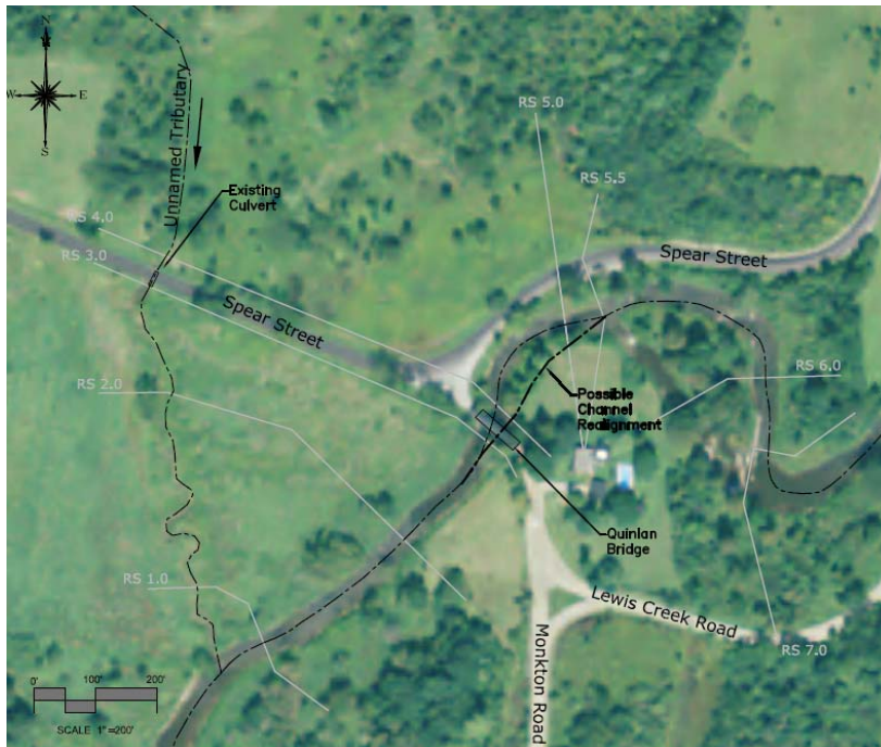
Figure 31: Alternative schematic of channel realignment upstream of Quinlan Bridge.
