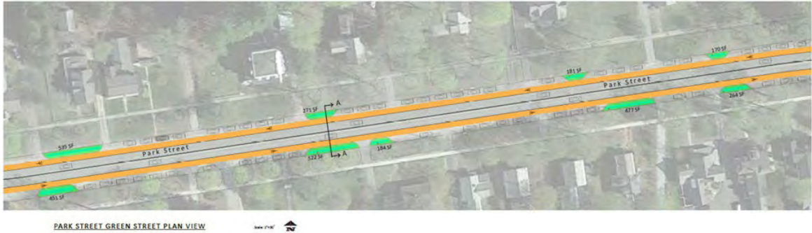
Figure 30. Park Street Green Plan Conceptual Design. Green = targeted areas for installation of bioswales upgradient from drop inlets to better infiltrate stormwater runoff.
