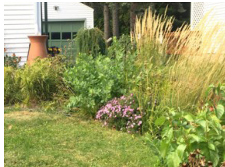
RAIN GARDEN. Captures runoff from areas such as rooftops, driveways, or parking lots. Slows, filters, and infiltrates runoff while irrigating plants in the garden.
