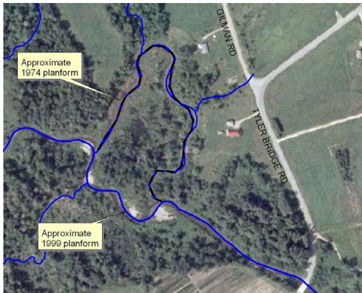
Figure G-19. Abandoned meander downstream of the Tyler Bridge Rd bridge in Segment M15-B. Review of annual fly-over images at the NRCS Middlebury office indicates that this avulsion occurred over a period of time from 1994 to 1995. Cut off of this broad meander resulted in a net loss of 1,000 ft of channel length. The avulsion and subsequent channel adjustments may have contributed to recent aggradation in downstream Segment M15-A. ( Base image is dated 2003)
